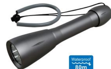
T-CY14-800 › Aluminum LED Diving Torch › Twist-on type › Brightness: 800 lumens › Battery: 3 x C battery (excluded) › Size: 228mm (L) x 54mm (D)
