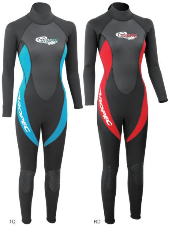
DS-5B07W-3/2mmF/N-TQ DS-5B07W-3/2mmF/N-RD › 3/2mm F/N Neoprene Fullsuit, Woman › 3mm Finemesh chest › 2mm Super-Stretch armpit & back waist › Other parts 2mm N/N Neoprene › Skin seal & adjustable neck › Back zipper & Flatlock stitched › Reinforced printed kneepad
